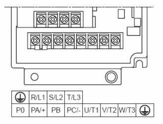
Motor and Power Terminal strip inside inverter
