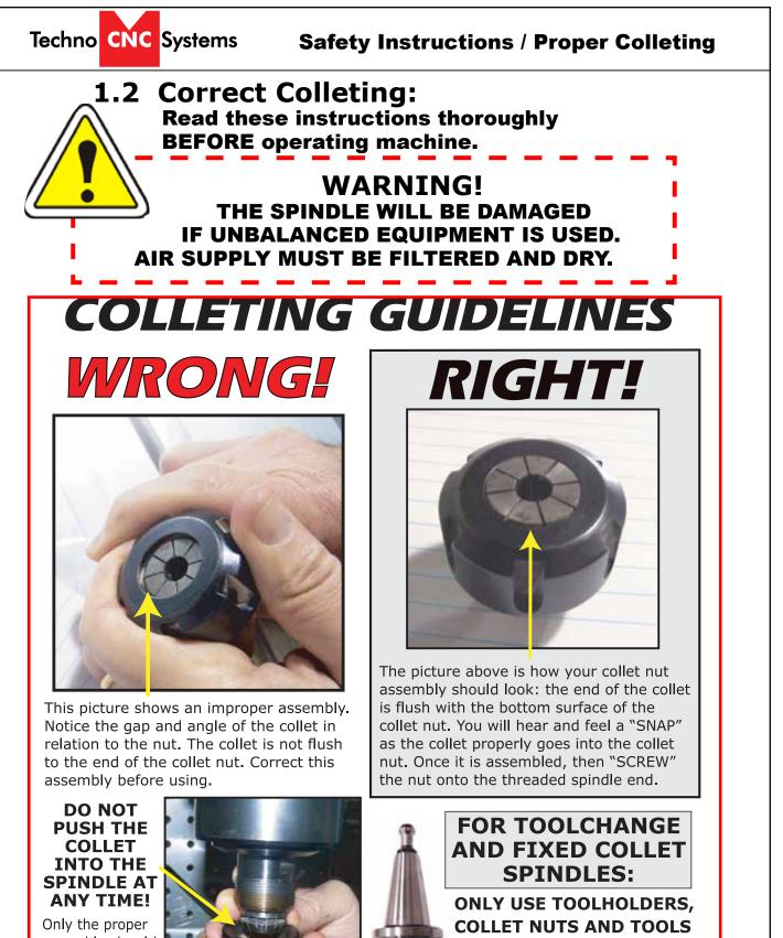
assembly should be screwed onto the spindle.
