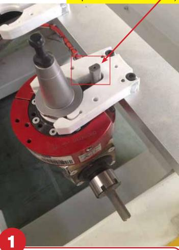
Diagram 1 illustrates how the aggregate must be seated in the ISO30 tool clip.
