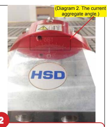
Diagrams 2 and 3 illustrate how to adjust the angle of the aggregate cutting tools.
