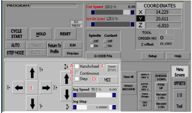
The machine will not move unless a jog mode is selected. Click on the button beside the text to select a mode.
