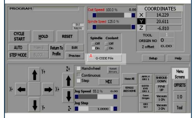
**A-G-code File:** Pressing this button will open the g-code file folder, allowing the user to activate or diactivate a g-code file.
