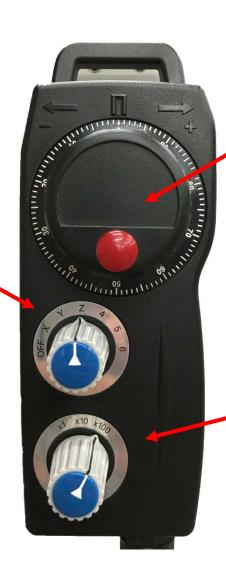
This knob is used to move the selected axis. Spin the knob clockwise to move in the positive direction. Spin the knob counter-clockwise to move in the negative direction.
