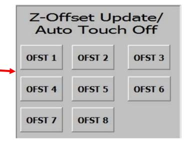
If you had identified the tool in the spindle as tool number 4, you will then choose "OFST 4". This will cause the machine to measure the length of tool 4 (currently in the spindle). The HDS will move to the touch-off probe and measure twice. The value will be saved as the Z-Offset for tool number 4. Press "Reset" to get rid of the blue notification.
