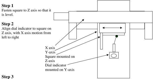
Loosen screws on bottom of extrusion holding Y-axis. Align Y- axis (in/out axis) w.r.t. square as Y axis moves in and out.
