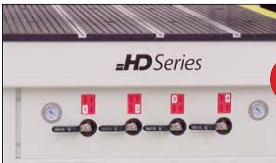
Turn on individual sections of the vacuum table by turning the manifold handles in the front of the machine.
