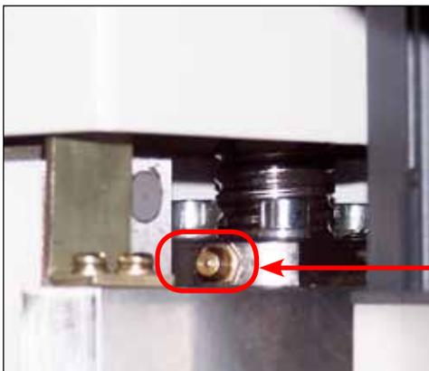
Lithium grease is pumped into the lubrication point with the application gun provided with the machine.
