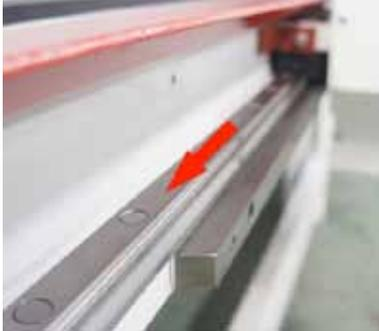
Lubricate the rack and pinion and the ball screw drive once every week so as to ensure longer service life.
