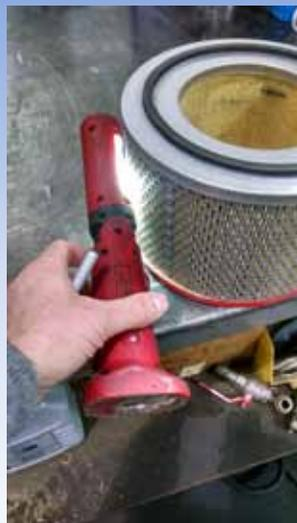
If light **cannot** be seen on the inside, the filter is clogged and needs replaced.
