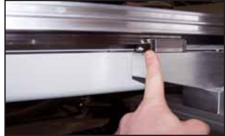
PICTURE 3: Gantry Grease Fittings
