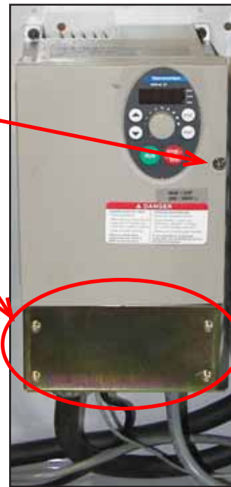
PICTURE 5: AC Spindle Motor Inverter
