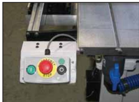
PICTURE 8: Mounted Start/Stop Box
