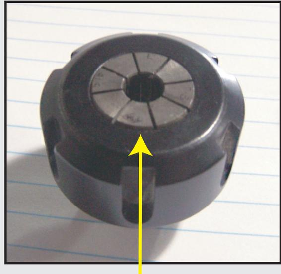
The picture above is how your collet nut assembly should look: the end of the collet is flush with the bottom surface of the collet nut. You will hear and feel a "SNAP" as the collet properly goes into the collet nut. Once it is assembled, then "SCREW" the nut onto the threaded spindle end.
