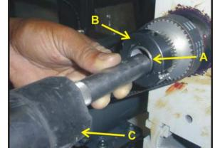
**Step 4:** (This IS necessary) For both the tightening and loosening procedures, you will need to retighten both set screws (inner and outer) that you loosened in **Steps 1** and **2** (above).
