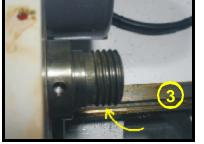
Step 3: Using a clean rag, wipe down and free the threads of any guck or debris.
