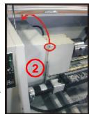
**ADJUSTMENTS:** Any adjustments to the spindle mechanism first require you loosen the two set screws (see pictures below)
