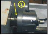
**Step 2:** Put a thick Allen wrench or bar into the hole left of the set screw you just loosened in Step 1. Leverage that bar against the base rail of the lathe while turning the chuck counterclockwise. Loosen the chuck enough to where you can unscrew it by hand (again, make sure the set screw is not impeding this process).
