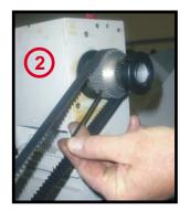
**Step 2:** Loosen the inner set screw. You may have to rotate the belt in order to gain access to the inner set screw (see picture at left).
