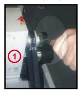
**Step 1:** Loosen the outer set screw (see picture at left).
